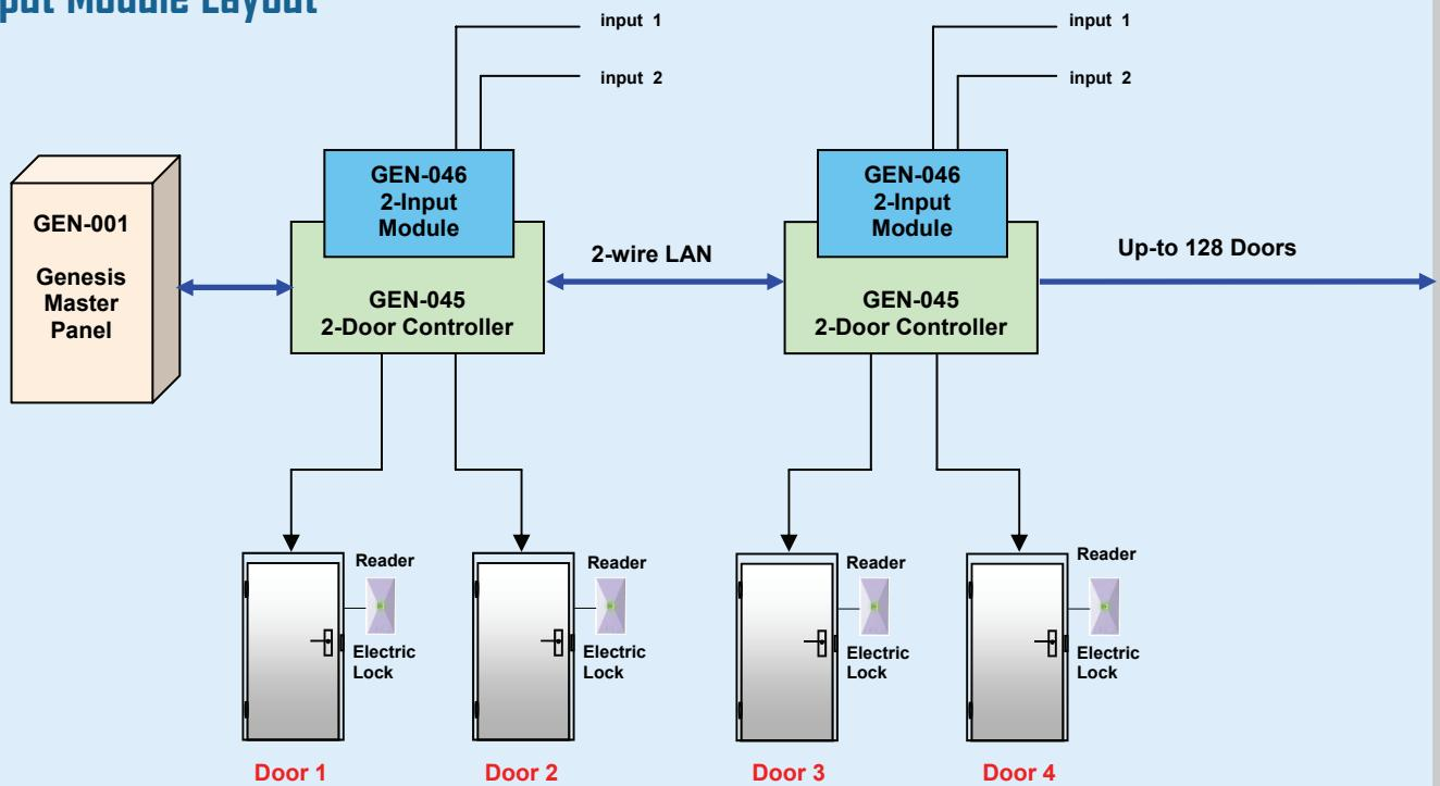
The 2-Input module can be used for additional door lock monitoring functions, or any other general purpose input applications
